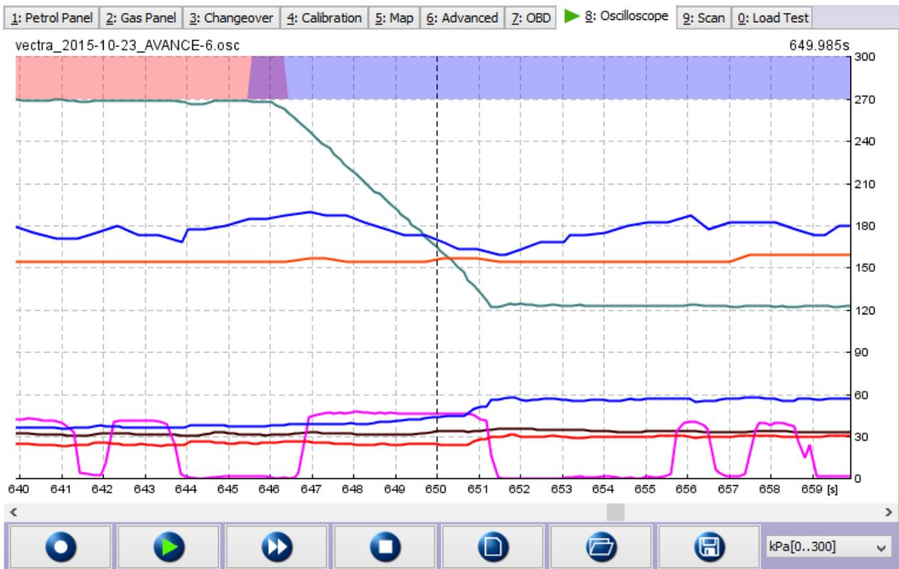
Oscilloscope shows run of selected ECU signals. On the right side of main window we can select (by marking a tick) which ECU signals we would like to see on oscilloscope run. We can also visualize required OBD readouts by selecting them from OBD icon located on the left side of the Toolbar.
